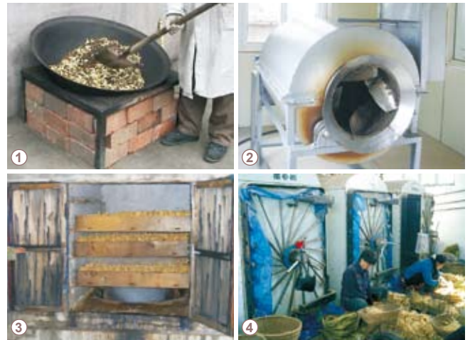
① Traditional frying wok ② Modern mechanized facility ③ Traditional steaming stove ④ Modern steaming equipment
